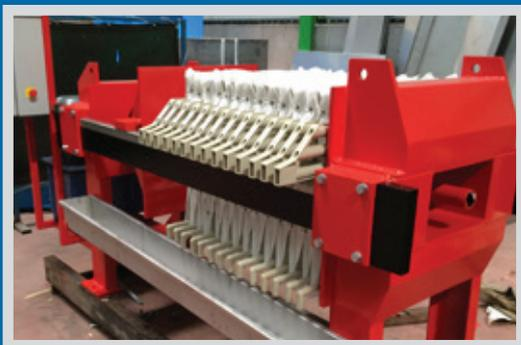
Filter Presses are dewatering equipments with the highest dewatering rate among all the mechanic dewatering equipments used. By transforming sludge like solid material into cake, the filter press separates water. Moreover, this kind of press is the most widely used dewatering system due to its economical and ease of use qualities.
