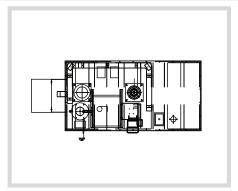
Polymer Dosing Units are mainly made up of tank, dry polymer storage reservoir, dry polymer feeding screw, rapid mixer, slow mixer and control panel.
